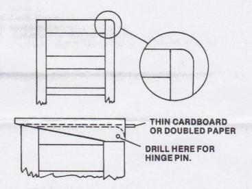
A. Round rear edge of chest assembly as shown. Place card-board or paper between lid and chest as shown. With back edges flush, drill holes in chest for the hinge pins. Insert pins partway in and check that lid opens and closes properly. Ad-
