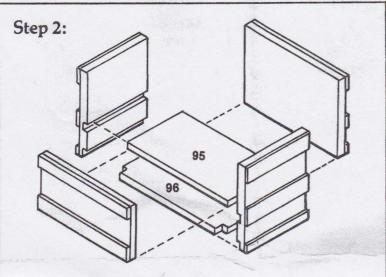
A. Glue center divider (95) and bottom (96) into the dadoes of sides (93) so that back edges are flush with the rear of the sides (93).
