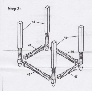
A. Glue the side spreaders (47) and front and rear spreaders (46) into the legs (48). Try all parts first since length of the dowels on the ends of the spreaders may need to be shor-
