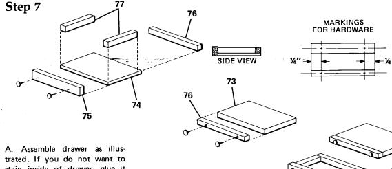
A. Assemble drawer as illustrated. If you do not want to stain inside of drawer, glue it together with white glue and finish front separately prior to assembly.
