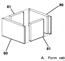
A. Form cabinet assembly by gluing sides (81) to front (80) and back (80). Top and bottom edges should be flush.
