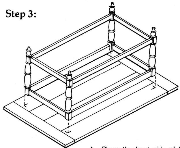
A. Place the best side of the table top made in Step 1 face-down. Align table base made in Step 2 and mark corners with a light pencil mark as an aid when gluing. Apply glue on top edge of base then glue base to top. Allow to dry and proceed with final finish.
