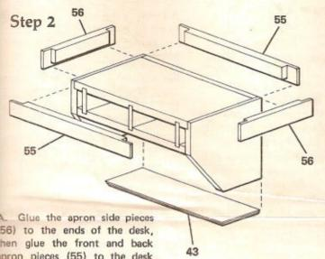
A. Glue the apron side pieces (56) to the ends of the desk, then glue the front and back apron pieces (55) to the desk and the end pieces. They should be centered so that they form a socket in each corner for the legs. Use a leg to check that they are spaced properly. Sand the outside corners smooth.
