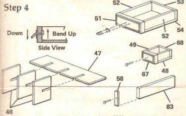
A. Glue the pigeonhole assembly together (Parts 46 & 47). Do not force the pieces or they may split. Sand to fit if necessary. Once it is dry, check its fit in the desk.
