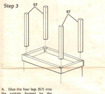
A. Glue the four legs (57) into the sockets formed by the apron. Square all of the legs and let the glue set before applying the final finish.
