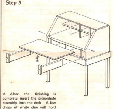
B. Install the knob and plate on the desk front (45) and then install the front by inserting the pins throught the holes in the sides. Re-drill the holes if they
