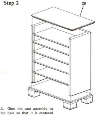
and the back edges are flush. B. Glue the top (26) to the case assembly so that it is
