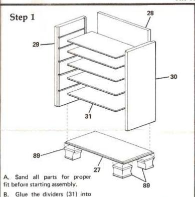
The fronts of the dividers should be flush with the extreme front edges of the sides. C. Glue the back (28) in place to align the entire case assembly.
