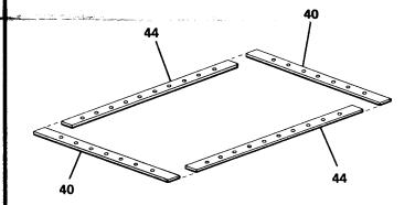
A. Utilizing Alignment Pattern No. 1, glue ends (40) to sides (44).
