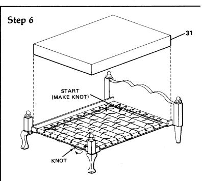
A. Repeat step 5 for stringing in opposite direction, weaving string over and under string installed in step 5.
