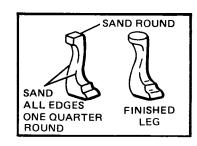
**NOTE:** Cabriole legs may be shaped prior to assembly, by sanding as shown.
