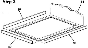
No. 2, glue side rails (39) and footboard (40)to frame assembly.
