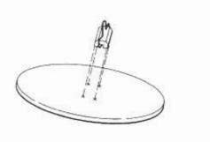
A. Locate center of top and place pivot block over center. Check alignment then lightly mark location. Glue into place.
